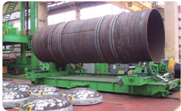
2 TURNING ROLLER & WELDING CAR SYSTEM
